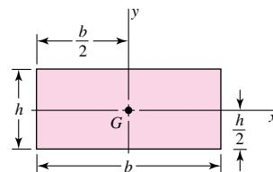
$$A = bh \quad I_x = \frac{bh^3}{12} \quad I_y = \frac{b^3h}{12} \quad I_{xy} = 0$$
