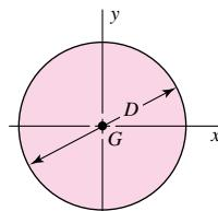
$$A = \frac{\pi D^2}{4} \quad I_x = I_y = \frac{\pi D^4}{64} \quad I_{xy} = 0$$
