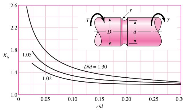
\*Factors from R. E. Peterson, "Design Factors for Stress Concentration," *Machine Design*, vol. 23, no. 2, February 1951, p. 169; no. 3, March 1951, p. 161; no. 5, May 1951, p. 159; no. 6, June 1951, p. 173; no. 7, July 1951, p. 155. Reprinted with permission from *Machine Design*, a Penton Media Inc. publication.
