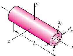
$$m = \frac{\pi (d_o^2 - d_i^2) l \rho}{4g} \quad I_x = \frac{m}{8} (d_o^2 + d_i^2) \quad I_y = I_z = \frac{m}{48} (3d_o^2 + 3d_i^2 + 4l^2)$$
