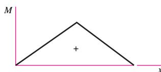
$$R_1 = R_2 = \frac{F}{2} \quad V_{AB} = R_1$$
