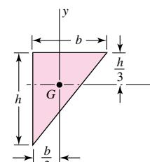
$$A = \frac{bh}{2} \quad I_x = \frac{bh^3}{36} \quad I_y = \frac{b^3h}{36} \quad I_{xy} = \frac{b^2h^2}{72}$$
