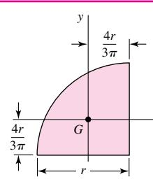
$$A = \frac{\pi r^2}{4} \quad I_x = I_y = r^4 \left( \frac{\pi}{16} - \frac{4}{9\pi} \right) \quad I_{xy} = r^4 \left( \frac{4}{9\pi} - \frac{1}{8} \right)$$
