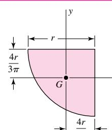
$$A = \frac{\pi r^2}{4} \quad I_x = I_y = r^4 \left( \frac{\pi}{16} - \frac{4}{9\pi} \right) \quad I_{xy} = r^4 \left( \frac{1}{8} - \frac{4}{9\pi} \right)$$
