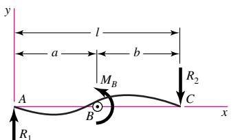
$$R_1 = R_2 = \frac{M_B}{l} \quad V = \frac{M_B}{l}$$
