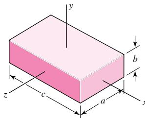
$$m = \frac{abc\rho}{g} \quad I_x = \frac{m}{12}(a^2 + b^2) \quad I_y = \frac{m}{12}(a^2 + c^2) \quad I_z = \frac{m}{12}(b^2 + c^2)$$
