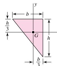
$$A = \frac{bh}{2} \quad I_x = \frac{bh^3}{36} \quad I_y = \frac{b^3h}{36} \quad I_{xy} = \frac{-b^2h^2}{72}$$
