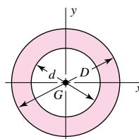
$$A = \frac{\pi}{4}(D^2 - d^2) \quad I_x = I_y = \frac{\pi}{64}(D^4 - d^4) \quad I_{xy} = 0$$
