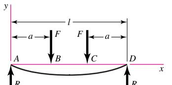
$$R_1 = R_2 = F \quad V_{AB} = F \quad V_{BC} = 0$$
