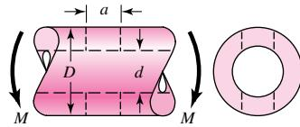
The nominal bending stress is  $\sigma_0 = M/Z_{\text{net}}$  where  $Z_{\text{net}}$  is a reduced value of the section modulus and is defined by
