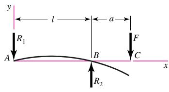
$$R_1 = \frac{Fa}{l} \quad R_2 = \frac{F}{l}(l + a)$$
